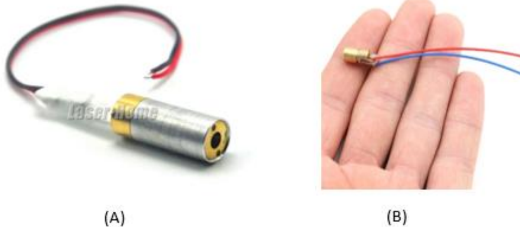
Figure 6: Semiconductor laser diode modules. A) Green laser. B) Red laser.
